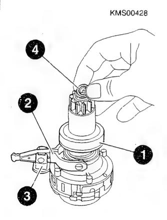
STARTING MOTOR ASSEMBLY Assembling overrunning-clutch drive Insert new snap ring in annular groove. ATTENTION: Take care not to damage output shaft.
